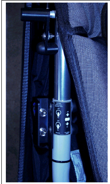
Figure 3 Section 2. Hand Throttle and Ignition Placard
