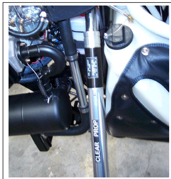
Figure 7 Section 2. Clear Prop and Fuel Spec Placards
