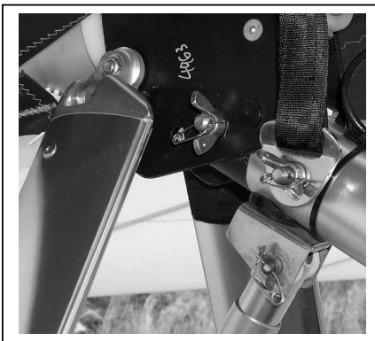
Figure 15 Section 4. Attach Wing to Wing U-Bracket
