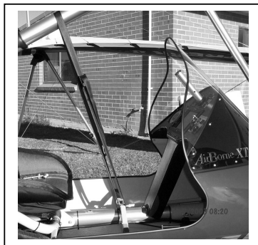
Figure 13 Section 4. Attach Mast Retaining Strap
