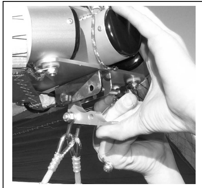
Figure 30 Section 4. Disconnect Nose Catch and Remove Nose Cone
