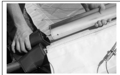
Figure 34 Section 4. Remove King Post
