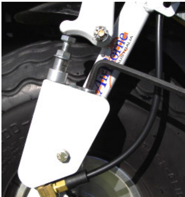
Figure 2 Brake master cylinder, remove reservoir plug
