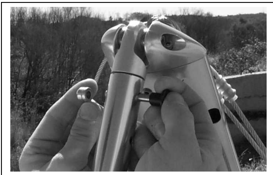
Figure 36 Section 4. Disconnect Base Bar
