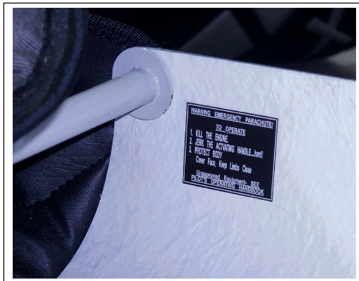
Figure 8 Section 2. Parachute Placard Location – (Pilots Left on Pod near to Seat Frame)
